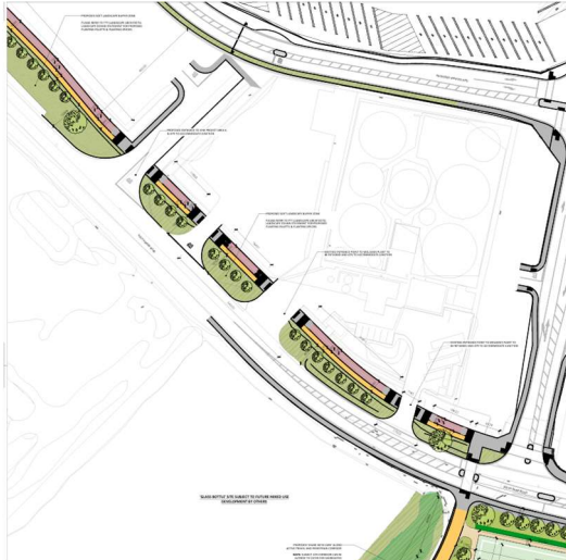
Fig. 105: Excerpt from the applicant drawings showing the number of dangerous entrances that cyclists must pass across (Source: Dwg. No. CP1901_011-DA-00-XX-DR-A-PA-006)
