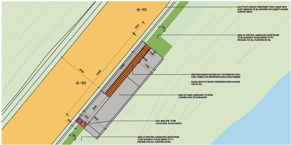
▲ Plan view of the 2no. proposed Intermediary Stop points proposed to the southern ATR corridor along Pembroke Cove
